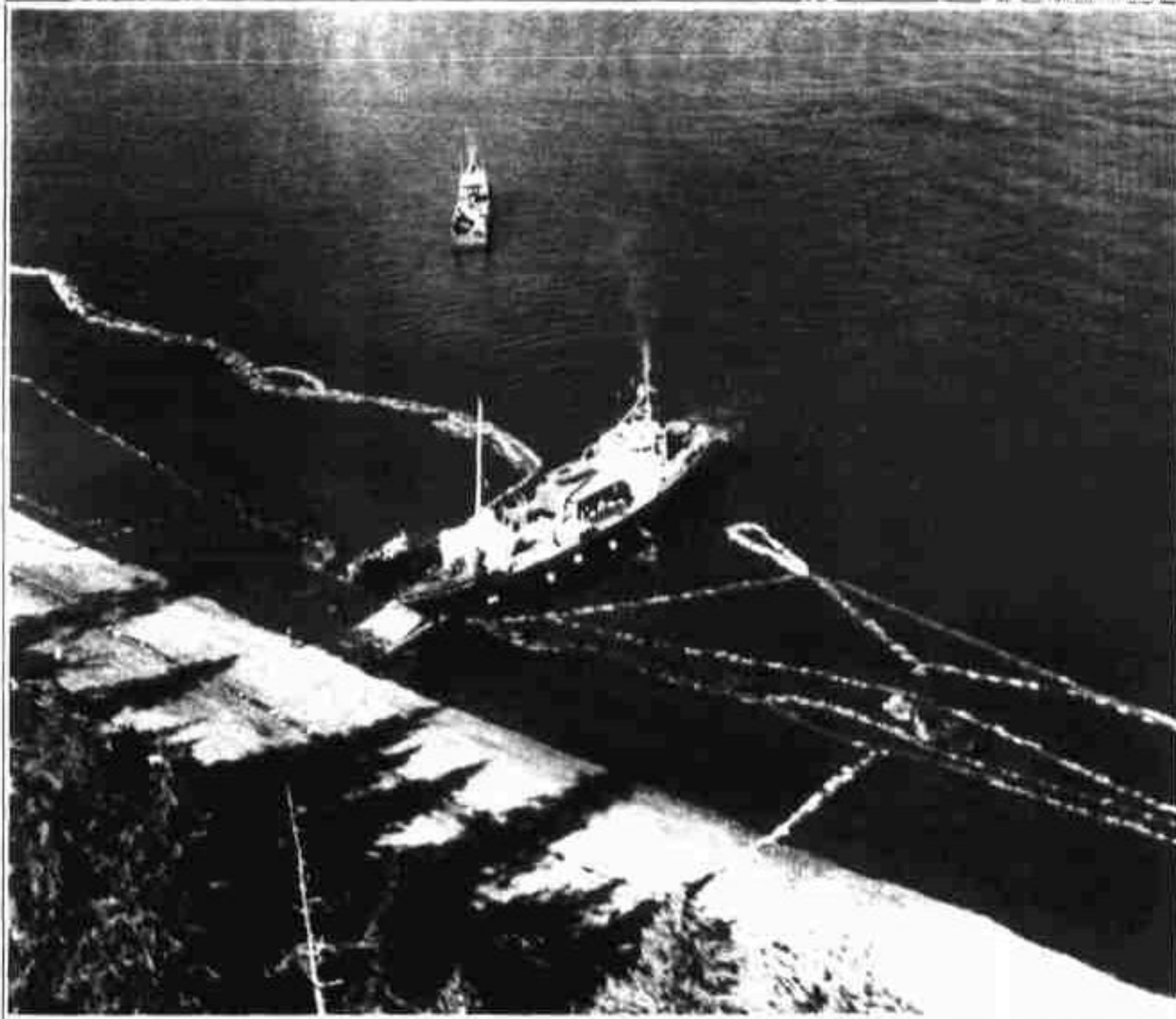
Oil spill clean-up work for 1990 is winding down in Prince William Sound. Above, containment booms are deployed at Sleepy Bay on LaTouche Island earlier this month. The vessel, the Glacier, is picking up heaving machinery used in the cleanup on the island this year.
