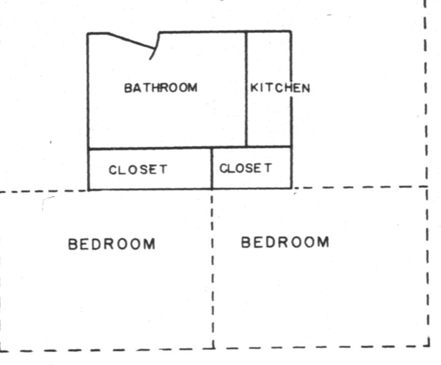
A TYPICAL housing plan that incorporates the Arctic Health Research Center's Bathroom-Kitchen Core Unit. The exterior dimensions of this house are 20' x 24'.
